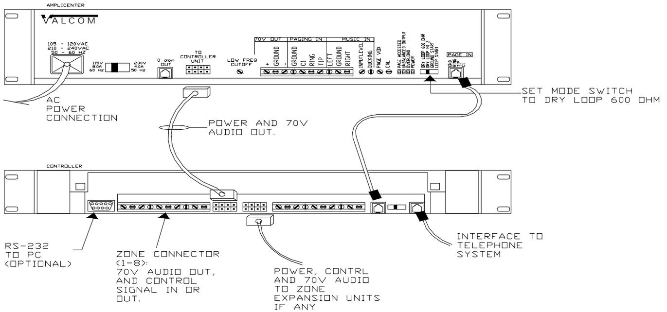
Figure 12. AmpliCenter Interface with PagePac Plus Controller (V-5323100)
