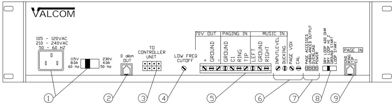
Figure 10. AmpliCenter Controls and Indicators, Terminals and Connector
