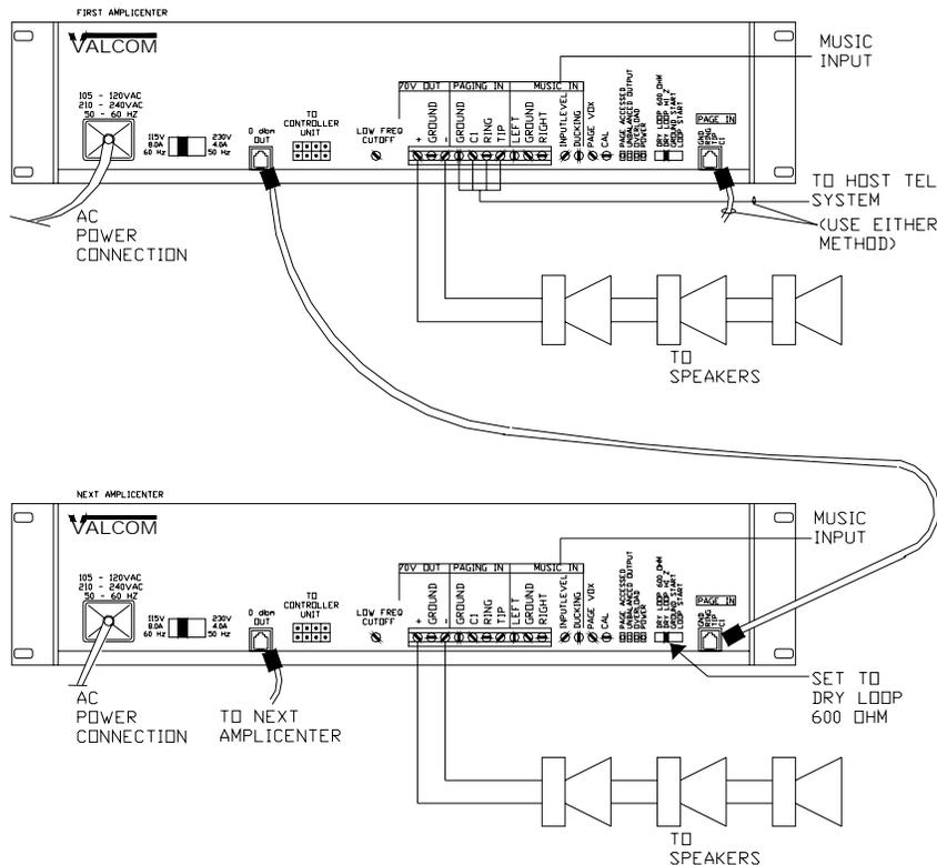
Figure 13. Series AmpliCenter Without Controller
