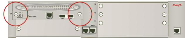
7 Tighten the captive screws on the S8300.
