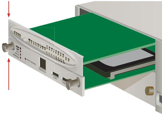
5 Align the LED module with the upper interior guides and insert until the faceplate is flush with the S8300 Media Server.
