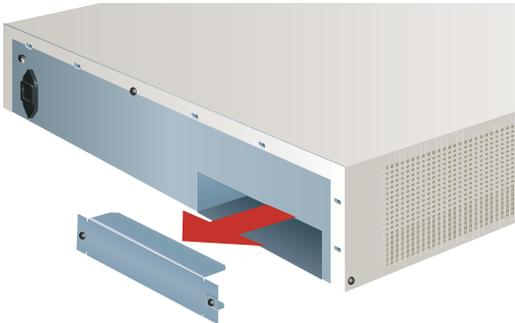
**1** Remove the blank faceplate from the Octaplane slot on the back of the media gateway.
