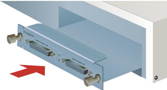
**2** Align the X330STK Octaplane Stacking Module with the interior guides and insert until firmly seated
